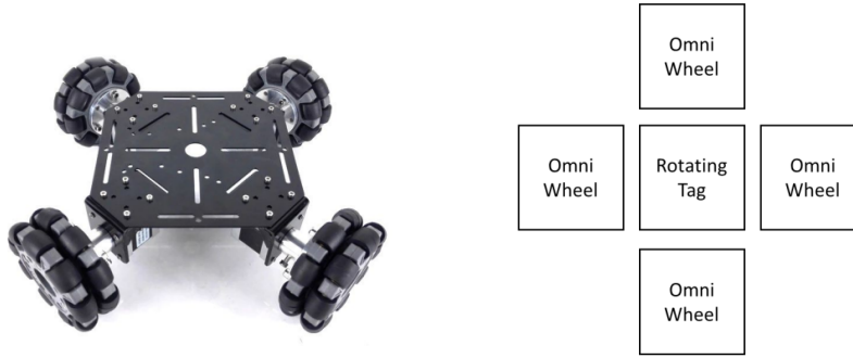
Figure 2: The schematic diagram of the holonomic robot
